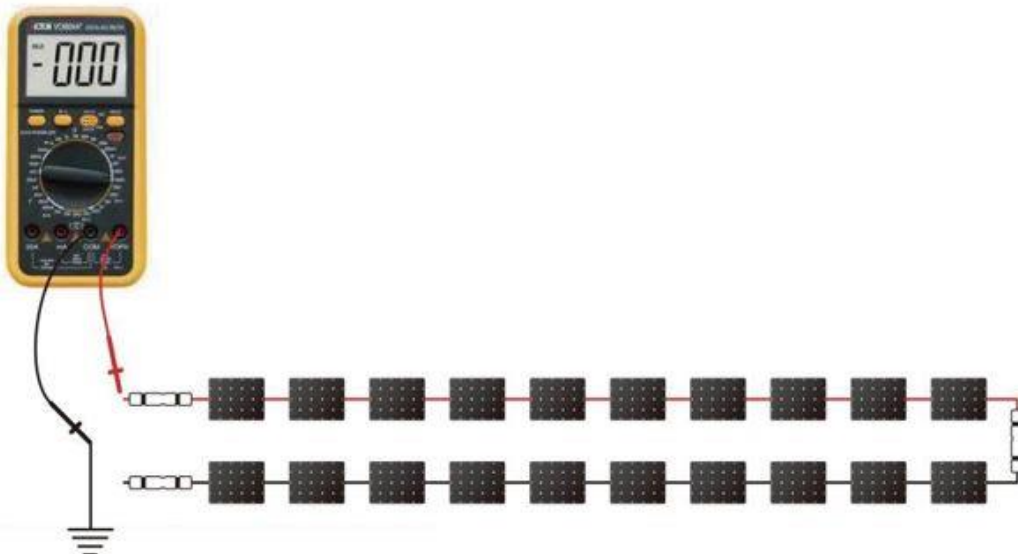
Figure 3-3 — PV String Cable Insulation Test [Error! Reference source not found.]
